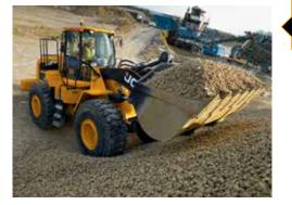
Class-leading climbing and stockpiling capability with high power-to-weight ratio and 27° departure angle. Z-Bar loader design delivers 188kN of breakout force.
