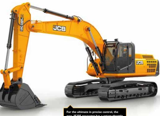
For the ultimate in precise control, the new JS305 excavator has a rotary throttle controller. There are also three work modes to tailor your machine to any application: Eco, Power and Power+.
