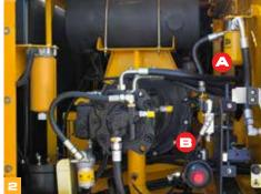
(A) Hydraulics oil filters (B) Fuel filters
